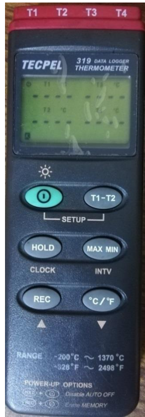
Figure 12: Data logger used
