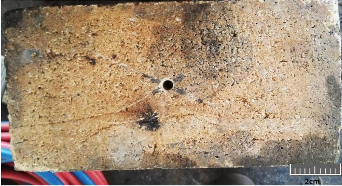
Figure 14: Fire brick for holding Sample
