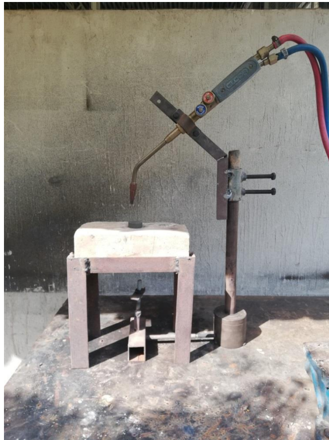
Figure 14: Fire brick for holding Sample
