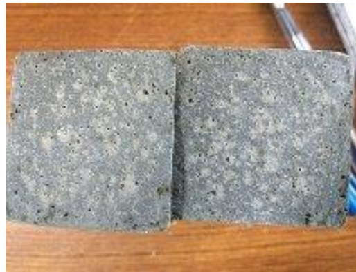
Figure 4.15: Cross Section of SCP in hardened state containing 1% Acacia Gum
