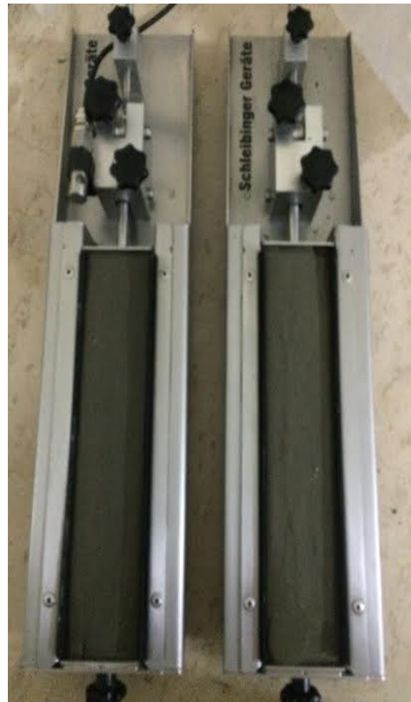
Figure 3.7: Shrinkage channels with sample
