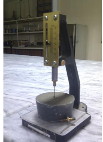
Figure 21 Vicat Apparatus Being Used for Final Setting Time
