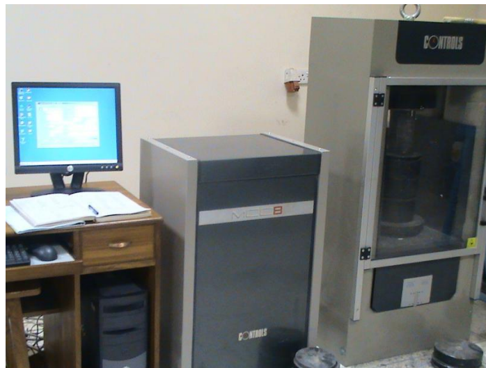
Figure 5.1: A Servo-hydraulic Computer Controlled Compression Testing Machine
