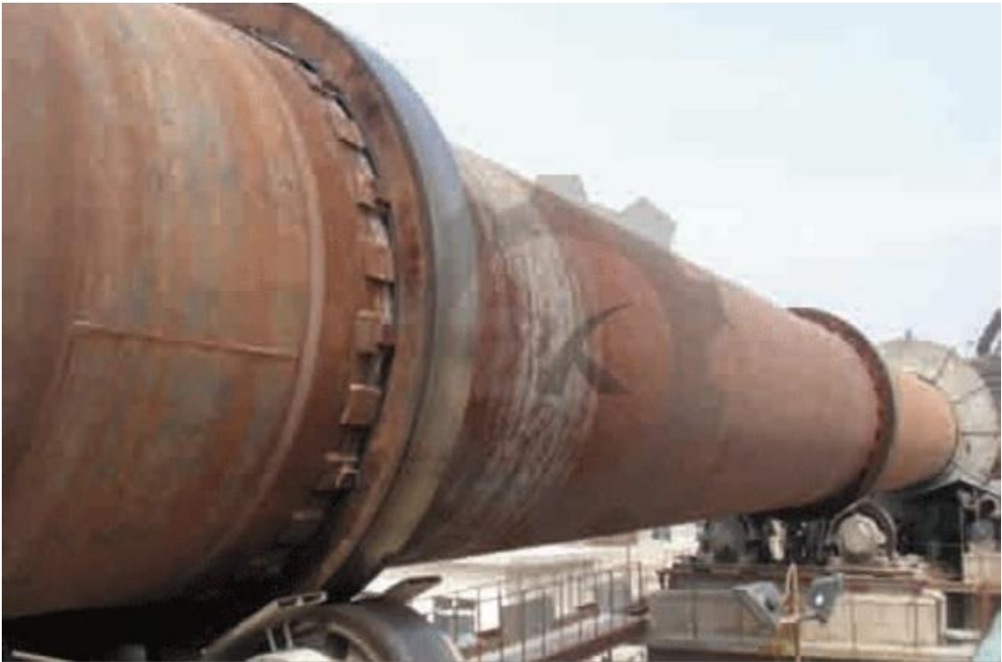
Figure 9: Rotary Kiln for Expansion and Bloating of Aggregates
