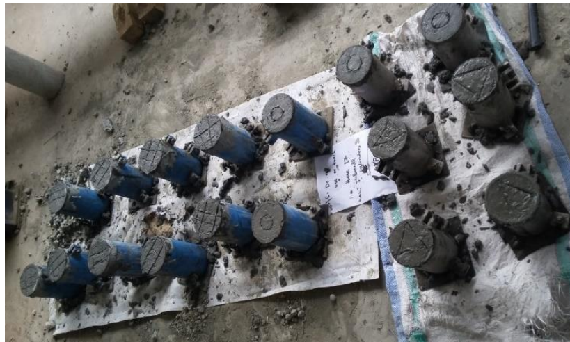
Figure 10: Casted Cylinder Samples of Fresh Concrete
