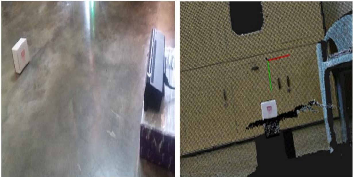
Fig. 7.3.1 Actual scene and its Point cloud (Box)
