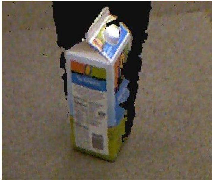
Fig. 2.6.1 Typical occlusion issues in a Point Cloud [8]
