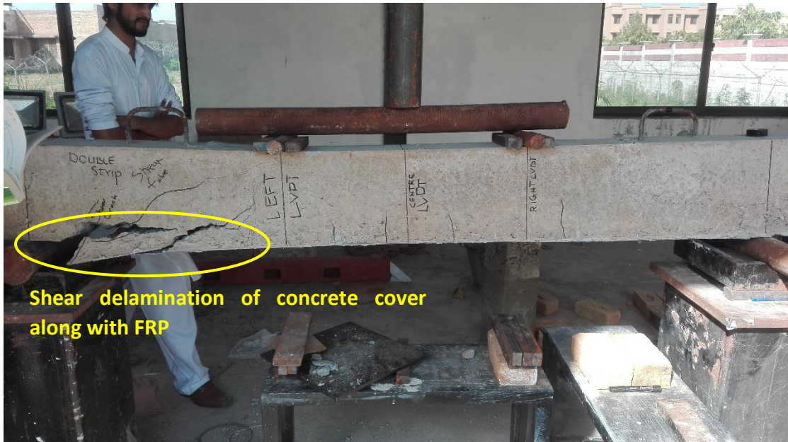
Figure 5-4: FRP double strip specimen failure
