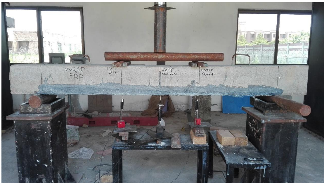
Figure 4-10: Loading configuration of the beams
