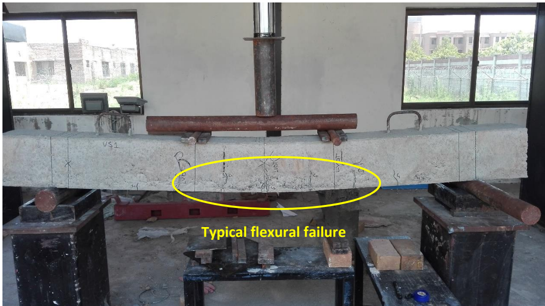
Figure 5-1: Reference specimen failure
