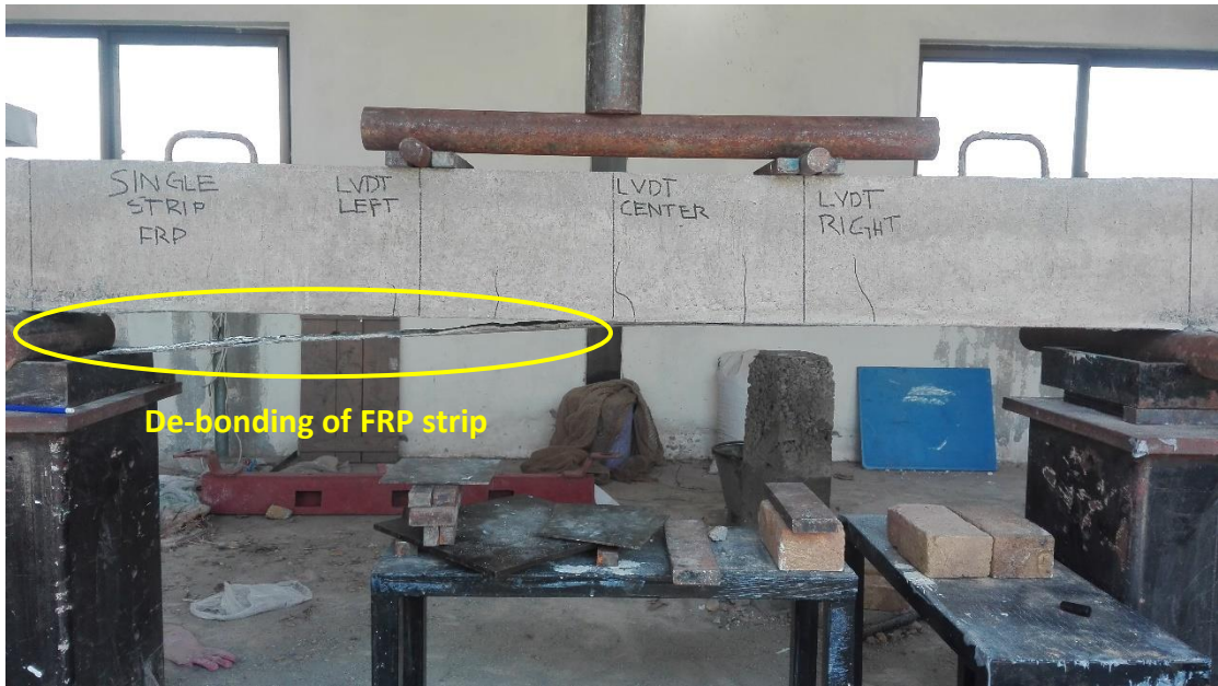
Figure 5-3: FRP single strip specimen failure
