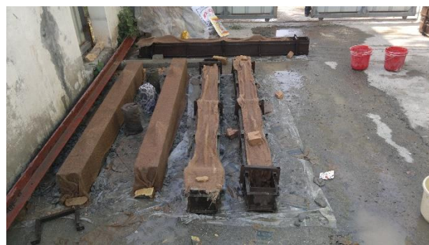
Figure 4-4: Curing of sample beams
