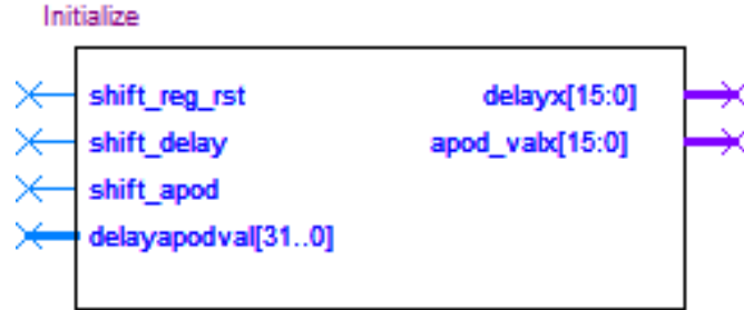
Figure 28 - Inputs/outputs of delay and apodization block
