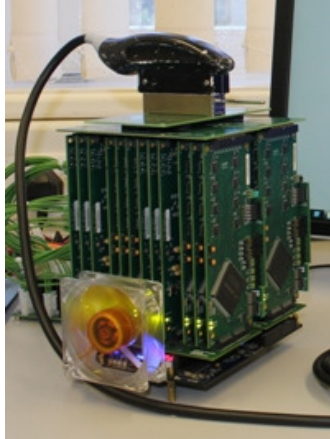
Figure 20 – UARP Tx and Rx circuit mounted on a STRATIX III FPGA board
