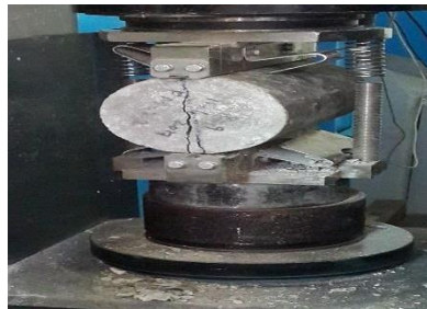
Figure-5 Split Tensile Test
