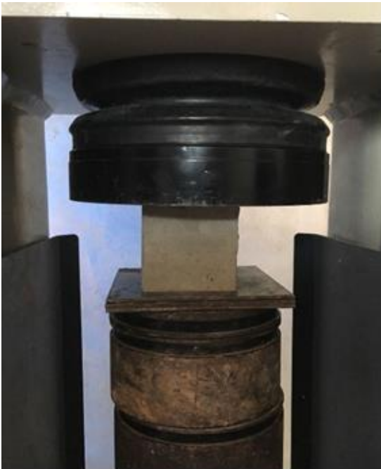
Figure 8 Cube being tested for Compression in Compression
