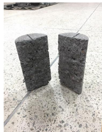
Figure 10 cylinder after split test
