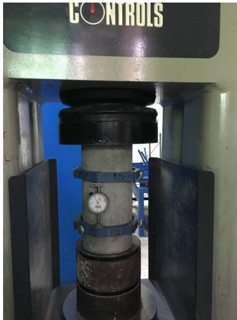
Figure 9 cylinder with assembly in compression machine
