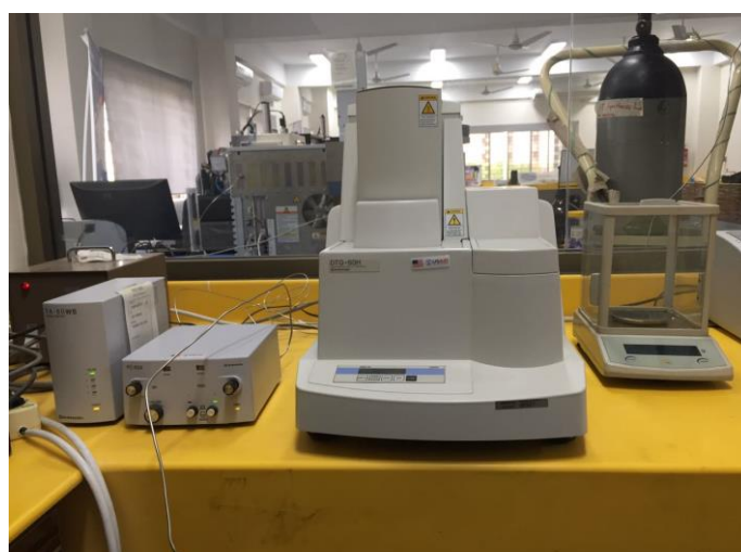
Figure 13 SHIMADZU Differential Thermal Gravimetric Analyzer (DTG-60H)
