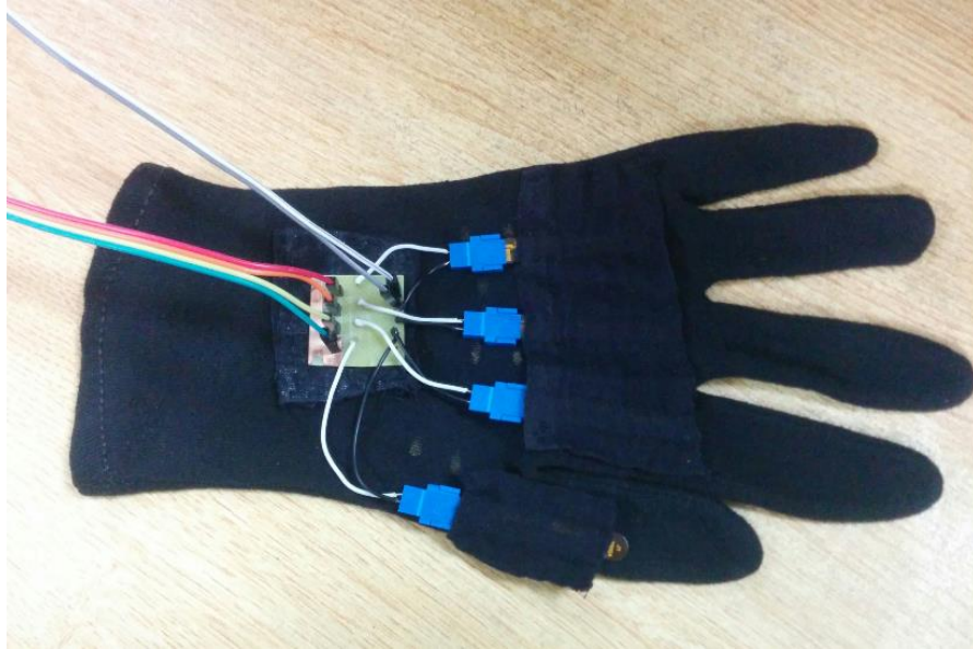
Figure 20: Flex Sensor Glove for accurate hand postures determination
