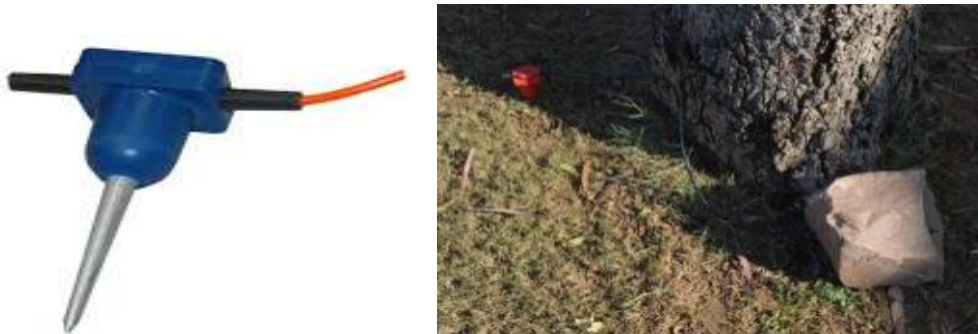
Figure 2.5: Seismic Sensor (Left) and Seismic Sensor installed with a fiberglass stone (Right)
