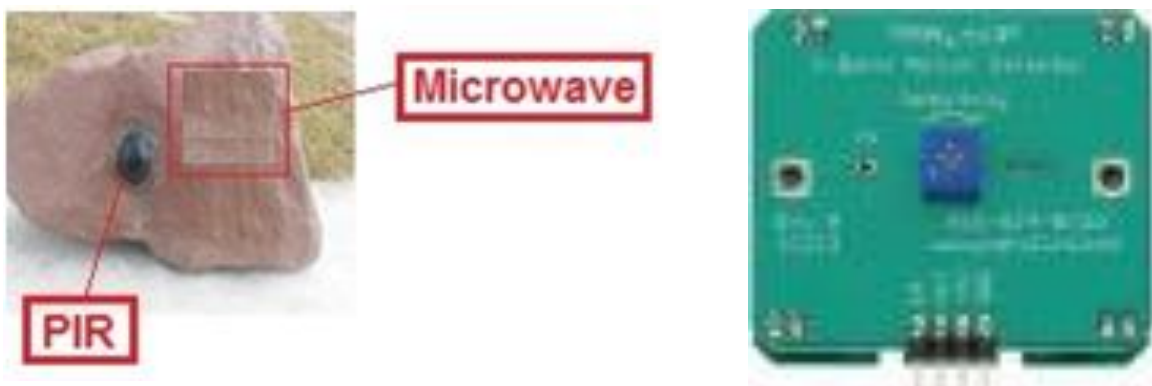
Figure 2.4: MW Sensor installed with a PIR in fiberglass stone (Left) and Microwave Sensor (Right)
