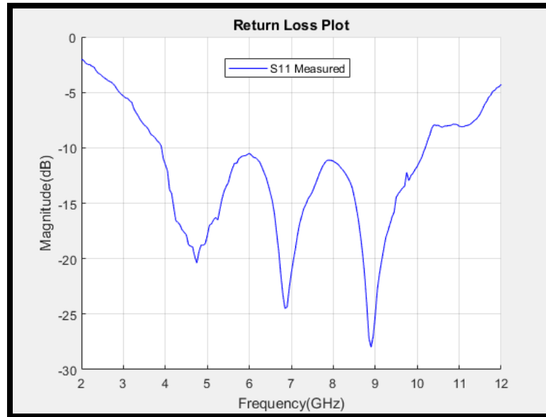
Figure 4- 5: Single Element with Stub and Slot (Measured)
