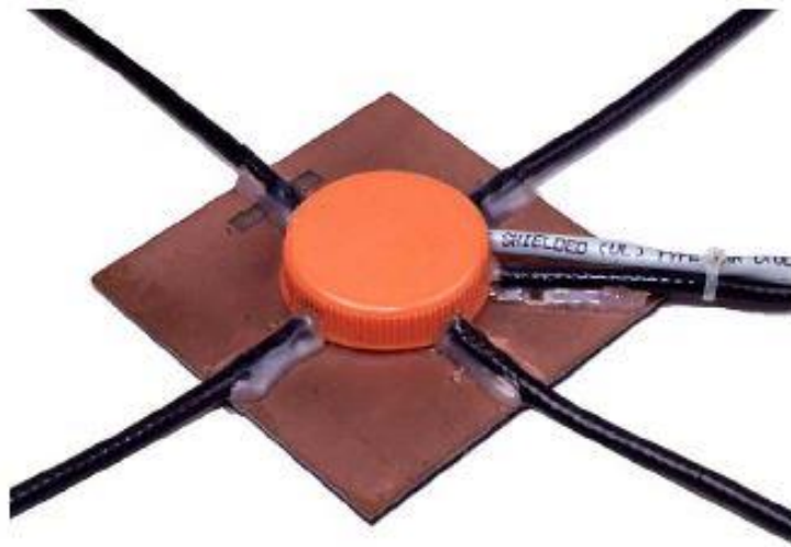
Figure 6 A close up of Antenna Switcher.
