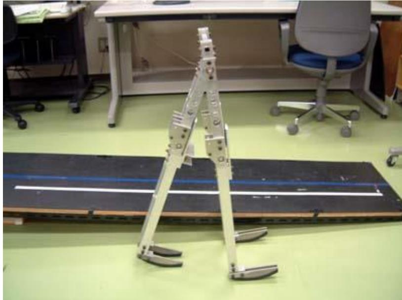
Figure 2.2 Passive Dynamic Walker Seno Laboratory, Nagoya Institute of Technology [61]
