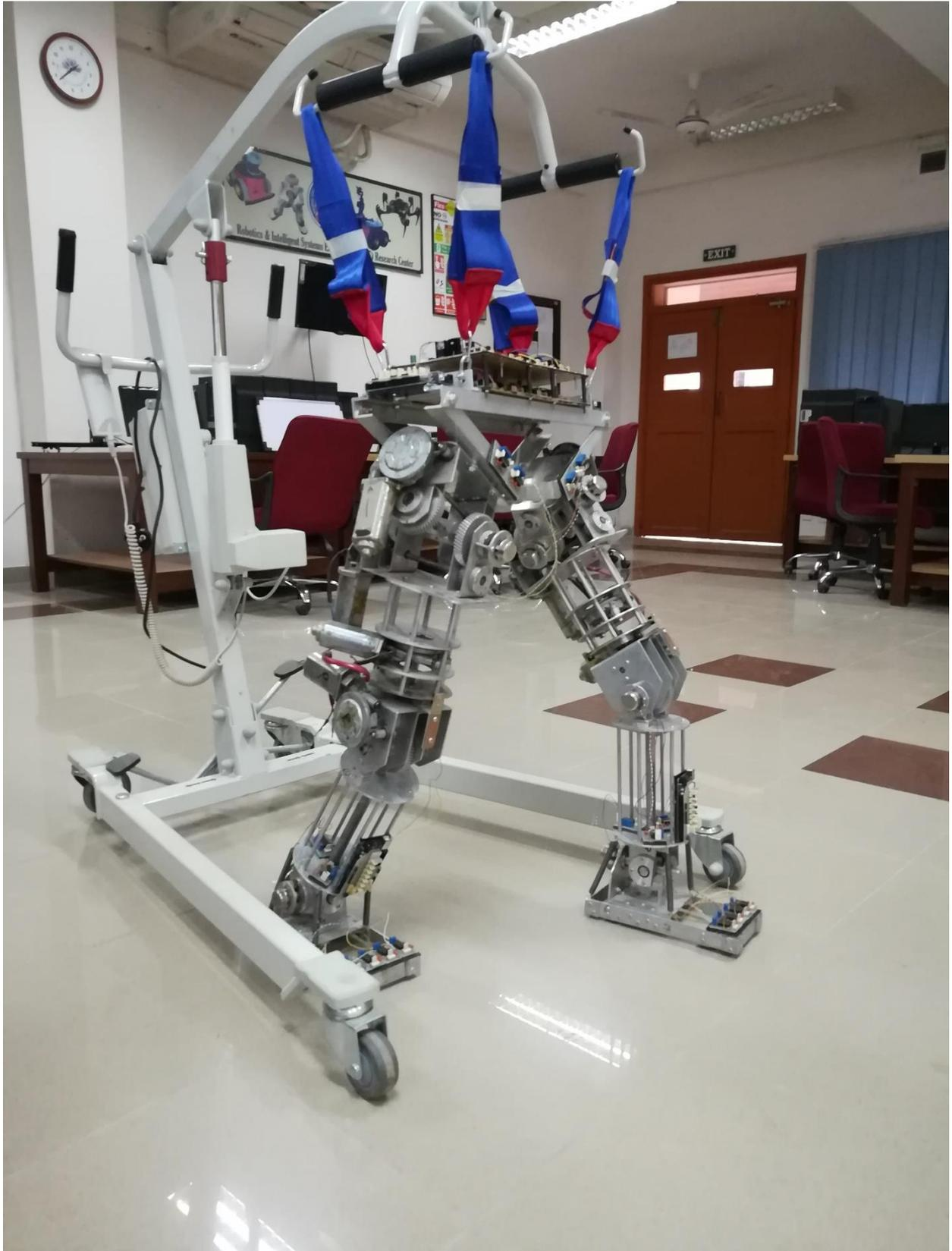
Figure 3.13 The Humanoid Robot NUSTBOT-3 Hardware Model with un-torqued ankles
