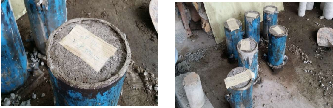
FIGURE 24 : CASTING OF CYLINDERS
