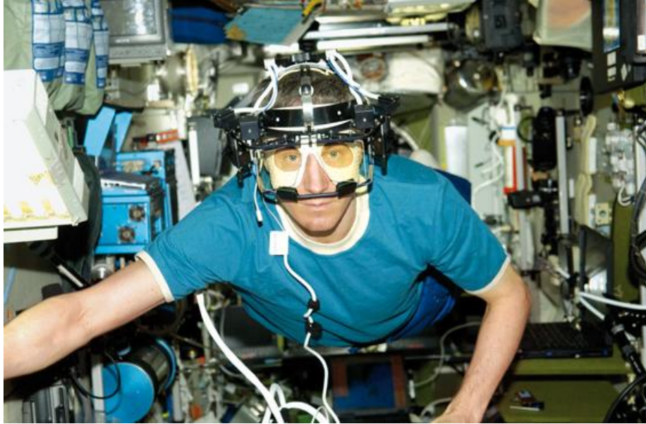
Figure 13. Mobile system for gaze tracking in zero gravity
