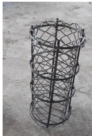
Figure 6 Reinforcement with GW Mesh
