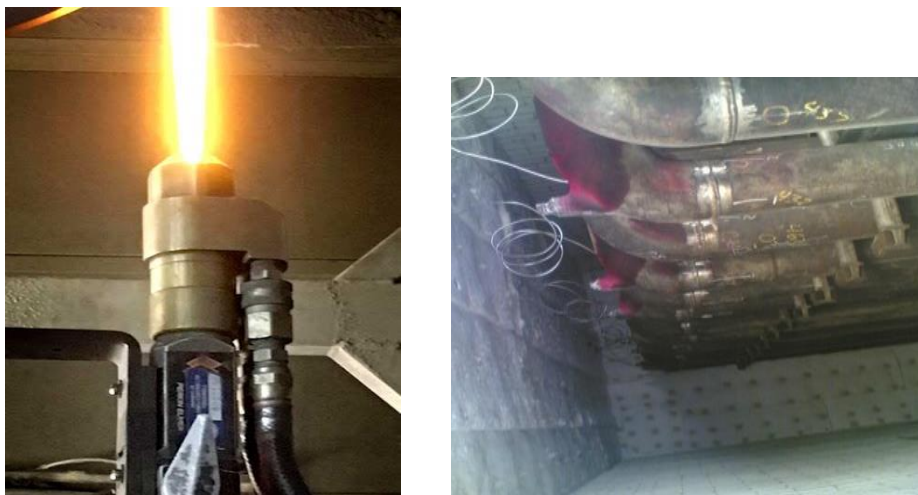
Figure 20: Needle Flame (Left) and Flame Impingement (Right)
