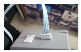
**Charging Pin** used for charging the microcontroller battery.
