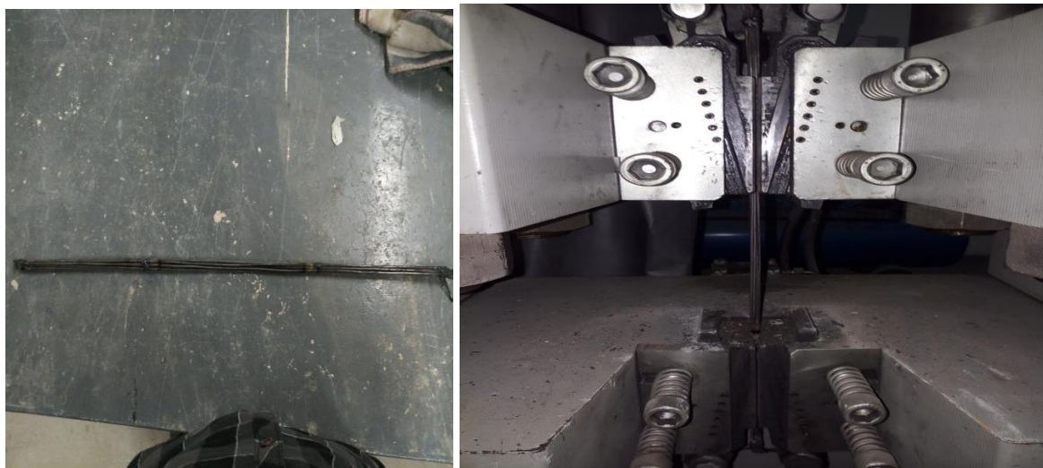
Figure 3.2: Model reinforcement undergoing tensile strength test
