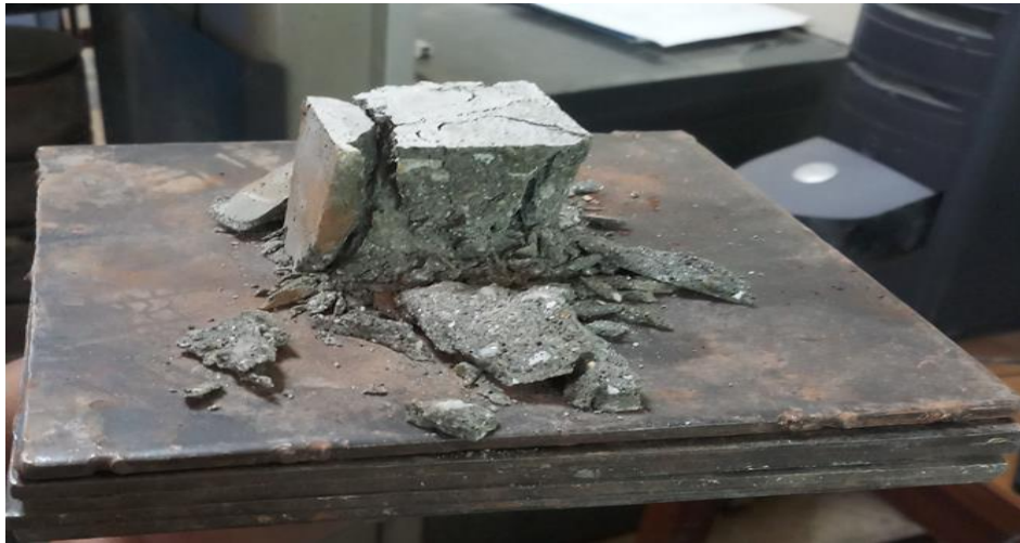
Figure 3.1: Concrete cube after compressive strength test
