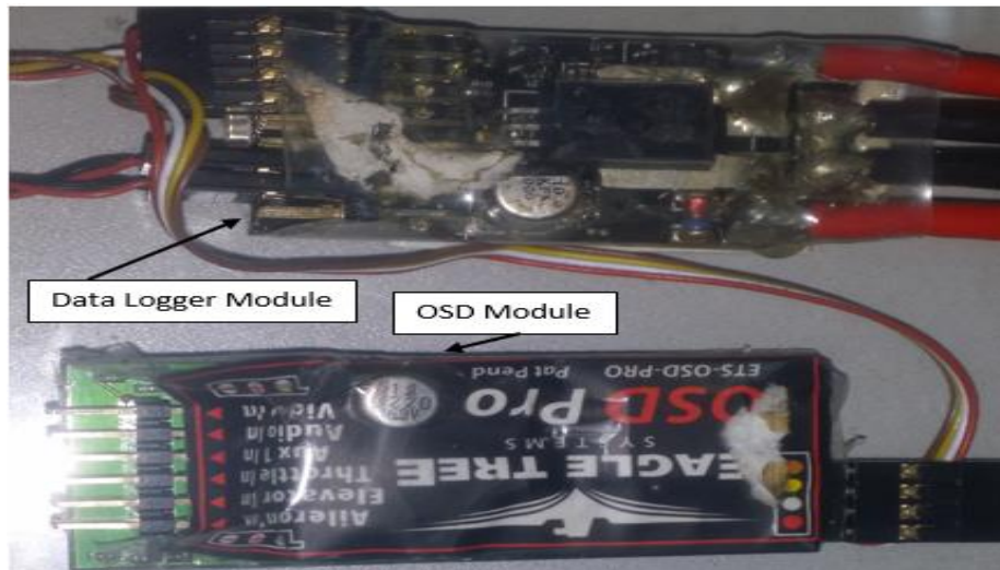
Figure 11.3: Connecting OSD module with the Data Logger Module.
