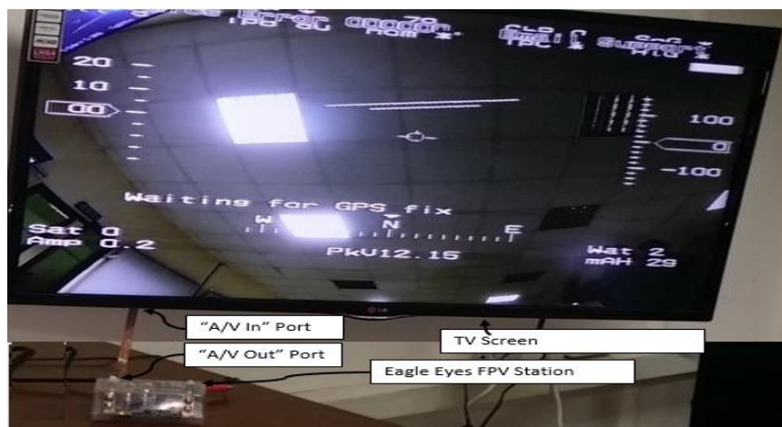
Figure 11.10: Connecting Eagle Eyes FPV Station with TV Screen.
