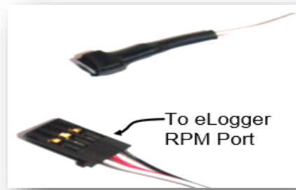
Figure 4.6: Port Description of the Eagle Tree OPT-RPM Sensor [16] .
