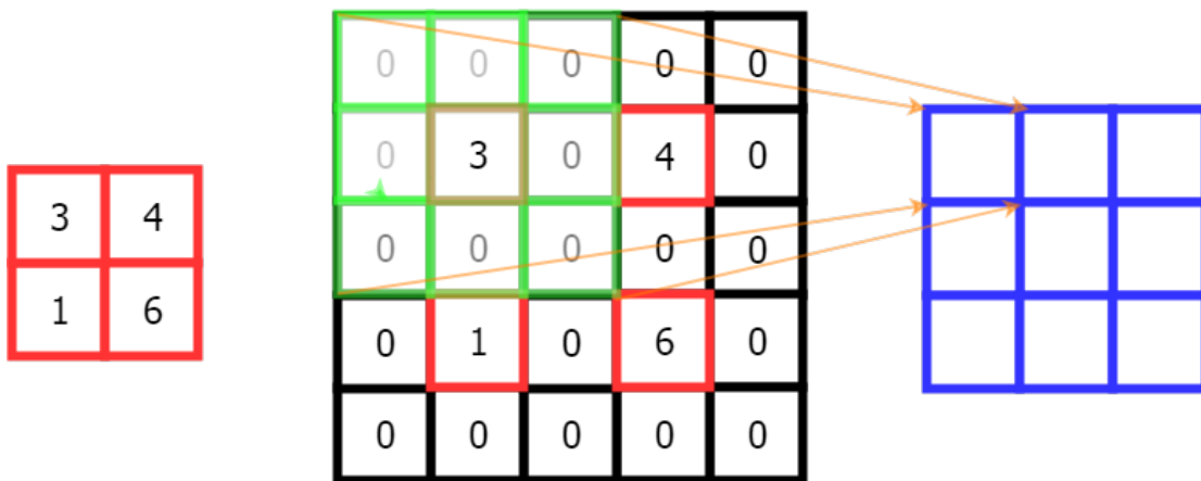
Figure 2.4: An example of the Fractionally Strided Convolution operation. The input feature map is shown on the left in Red. The middle image shows the zero-padded input image, with the convolution kernel shown in Green. The upsampled output is shown on the right in Blue.
