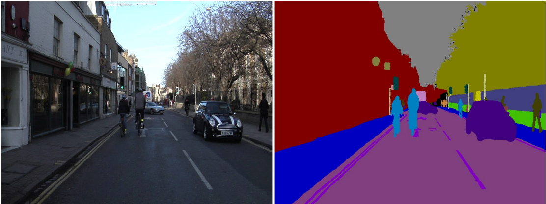
Figure 1.1: The Semantic Segmentation problem, where a mapping needs to be found from an input image (Left) to its Semantic Segmentation mask (Right) i.e. where all pixels are assigned to their respective categories. The example is from the CamVid dataset [1].
