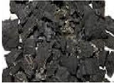
Figure 7: Raw pyrolyzed WT D_{50} = 1.27 \text{ mm}
