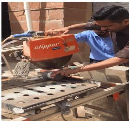
Figure 25: Sample preparation using diamond saw cutter
