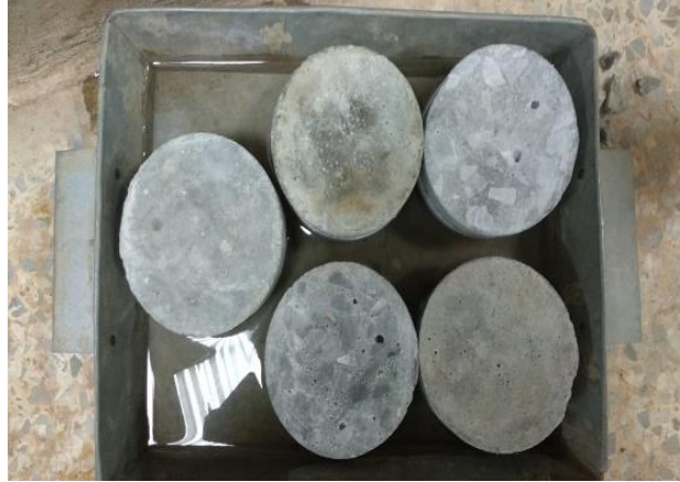
Figure 31: Concrete samples immersed in NaCl solution
