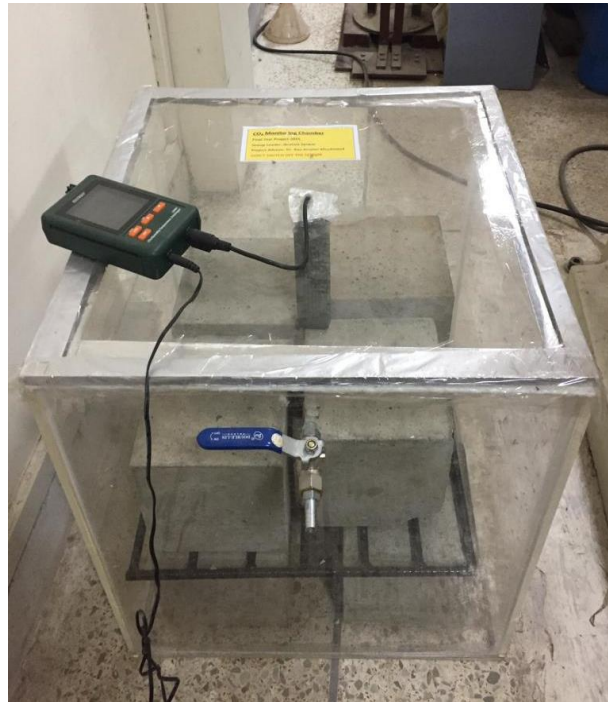
Figure 41: Real time CO 2 monitoring in the climate control chamber
