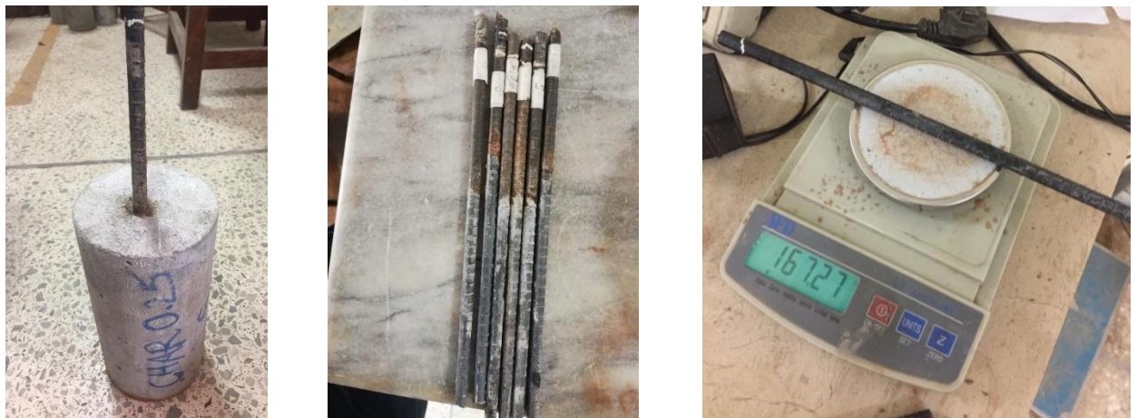
Figure 38: Pictorial description of weight loss measurement test
