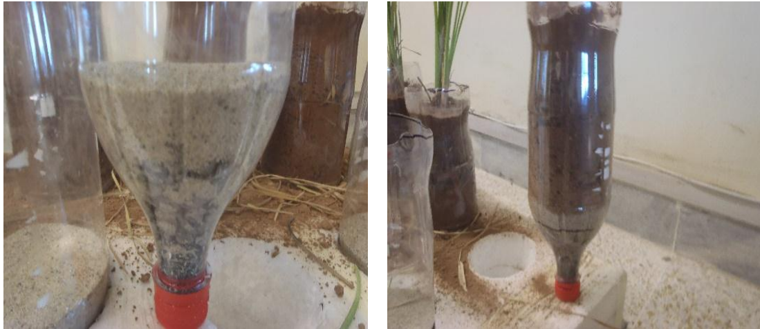
Figure 3.4 Constructed Wetland with the Fill Material
