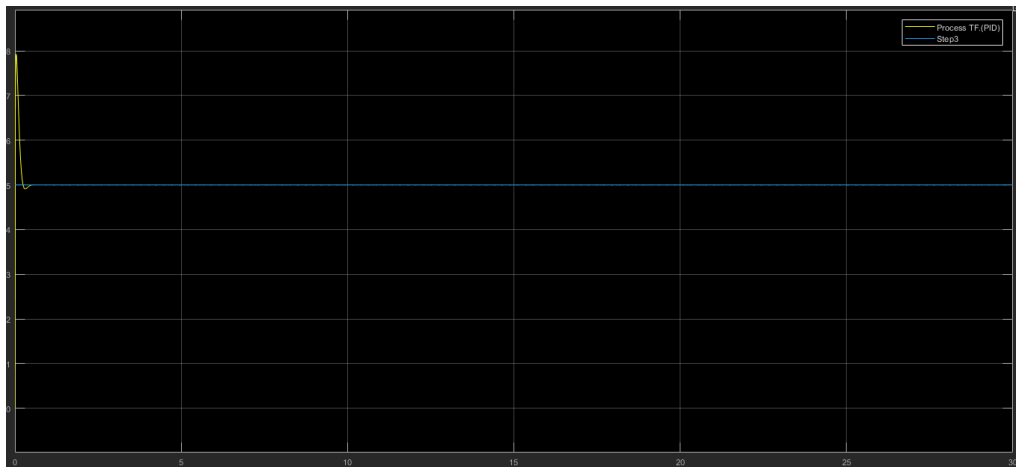
FIGURE 29: RESPONSE OF TEMPERATURE CONTROL LOOP TO STEP CHANGE
