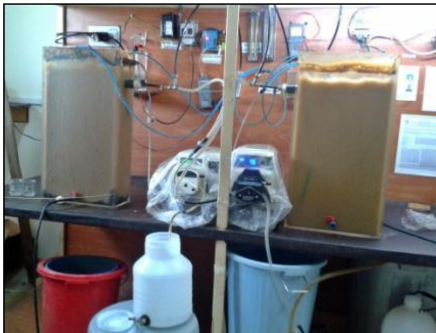
Figure 3.1: Membrane Bioreactor (MBR) at Water and Wastewater lab IESE
