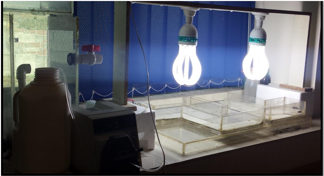
Figure 3.7: Bacterial Disinfection under Visible Light
