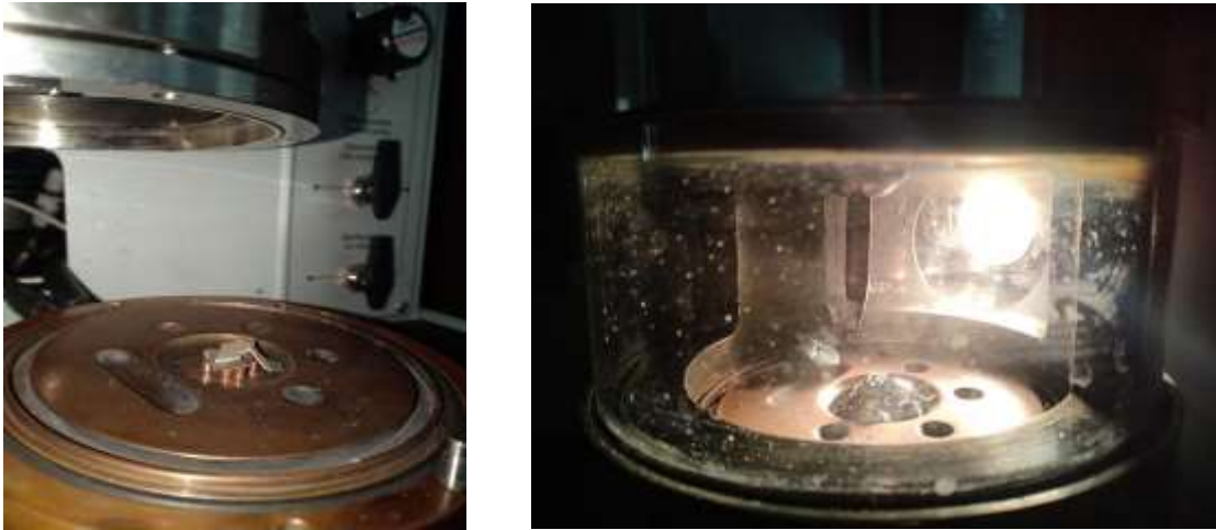
Figure 19: Layer by layer stacking of parent metals (left) closing the door of melting chamber and vacuum generation (right)
