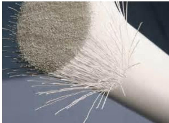
Figure 5: Hollow Fiber Membrane (0.05 > diameter)
