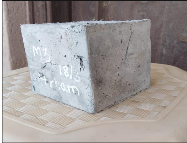
Figure 5.7: Post Failure Compressive test sample
