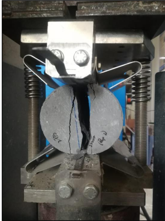
Figure 5.14: Abrupt Failure of mortar sample in split tensile test
