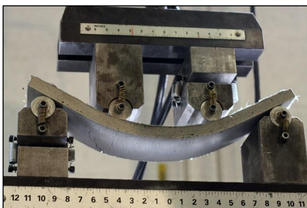
Figure 1.1: ECC under 4-point bend test. [1]
