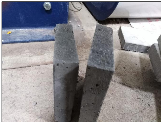
Figure 5.21: Abrupt failure of prism mortar sample in flexural test
