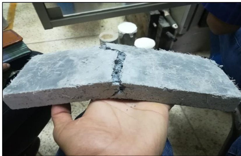
Figure 5.22: Ductile failure of ECC prism sample in flexural test
