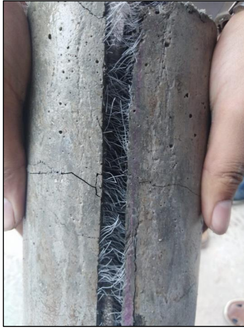
Figure 5.15: Ductile mode of failure of ECC sample in split tensile test
