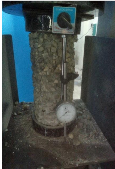
Figure 4 Specimen ready for testing with full set up
