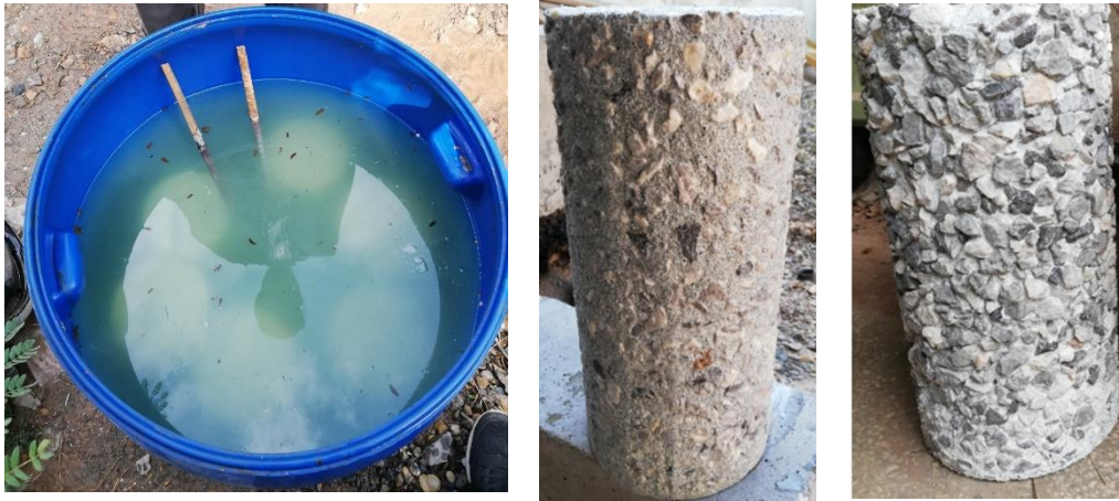
Figure 3 Sulphate medium and cylinders at 30 and 120 days exposure
