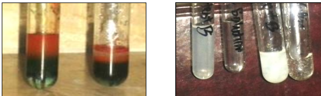
Fig 3.3 CMC chemical identification Test A and Test B (standard and local)
