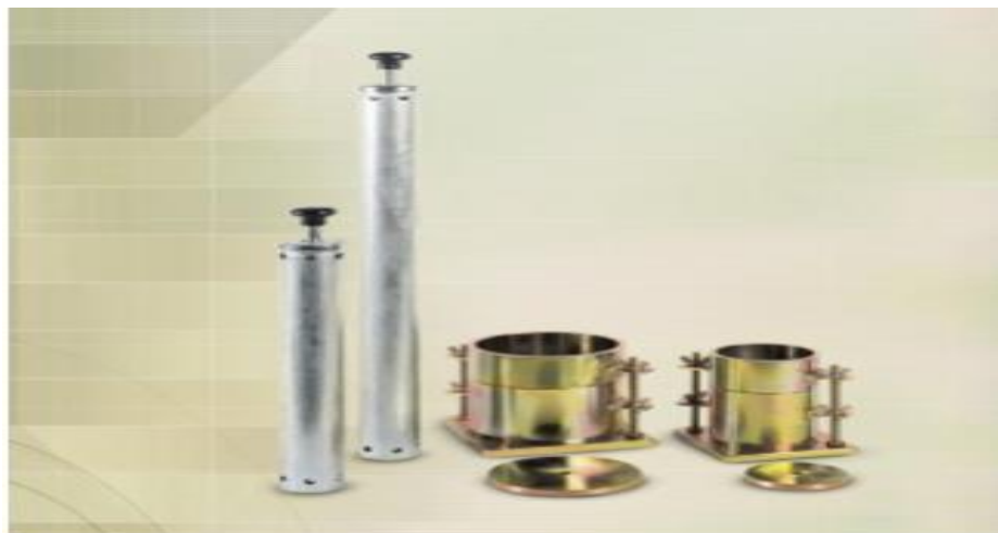
Figure 22. Assembly for Modified Proctor Test
