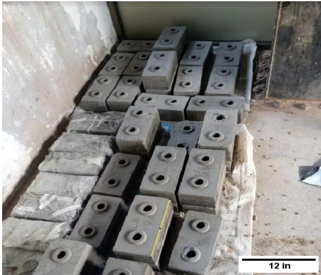
Figure 30. Compressed Earth Bricks left for Curing
