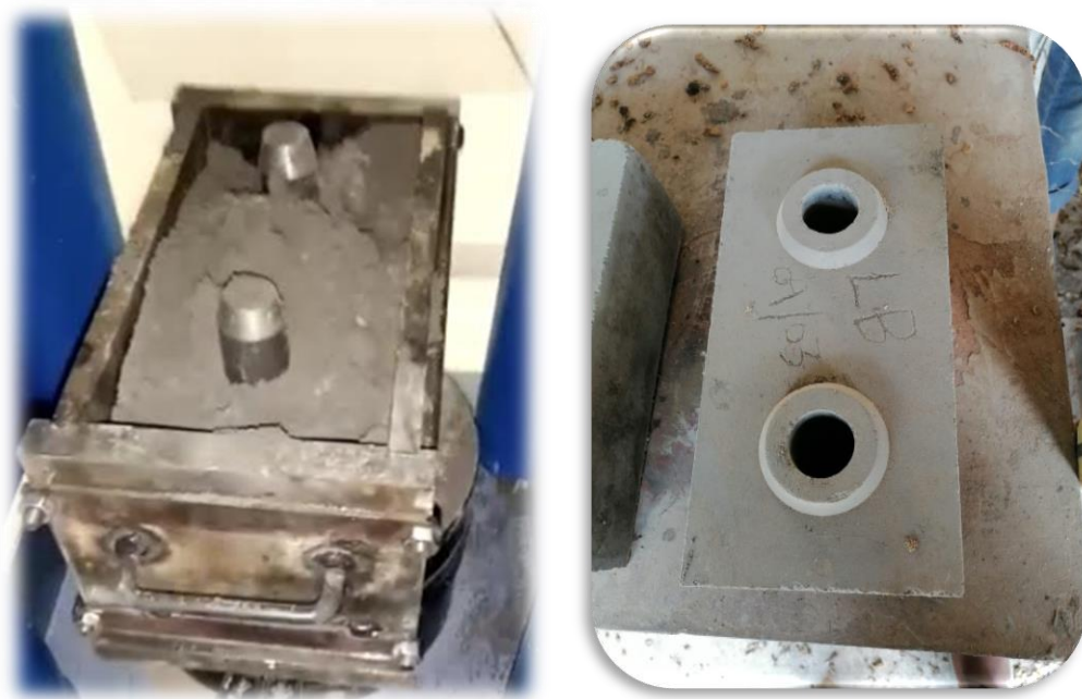
Figure 29. Compressed Earth Brick Extracted from Mold
